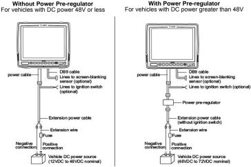
**CAUTION** Do not use the diode/choke assembly in the Extension Power Cable kit.
