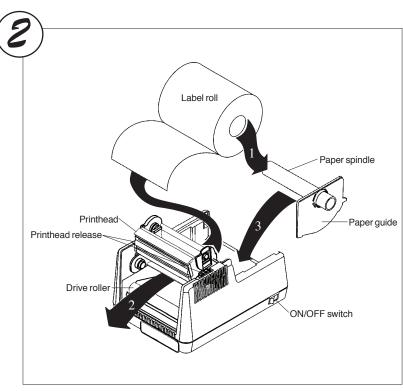
Thermal Transfer (TT) model shown. Printer is shown with media cover removed for clarity
