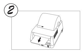
Release FEED button when printing begins. Printer will conduct a self-test and print a configuration label
