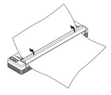
Carefully pull the paper out of the printer in either direction.
