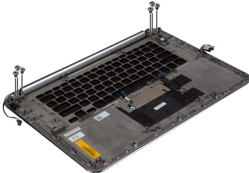
4. Lift the palmrest assembly away from the display assembly.
