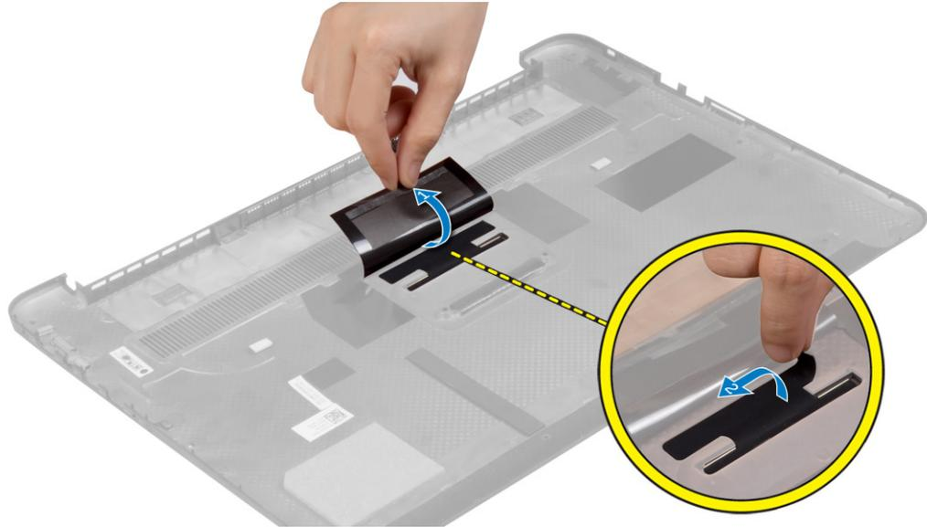
4. Release the tab on the system badge from the slot on the base cover. Lift the system badge off the base cover.
