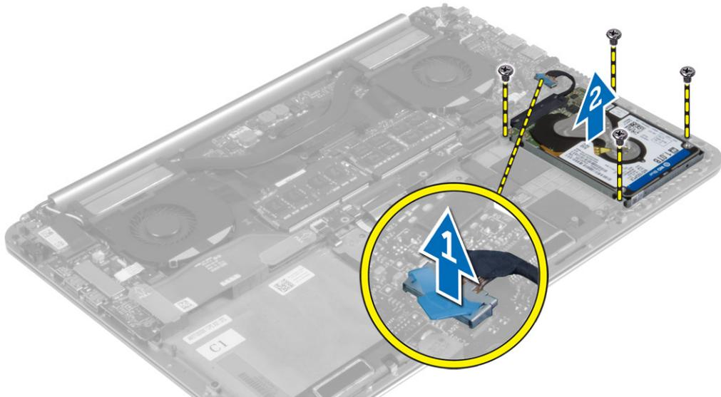
4. Perform the following steps to remove the hard-drive bracket:
