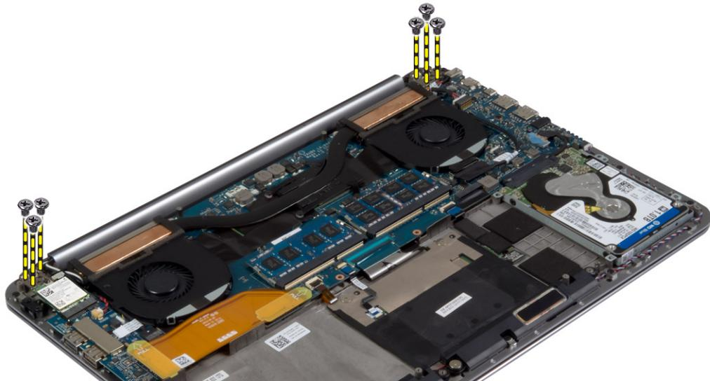
5. Lift and remove the palmrest assembly from the display assembly.
