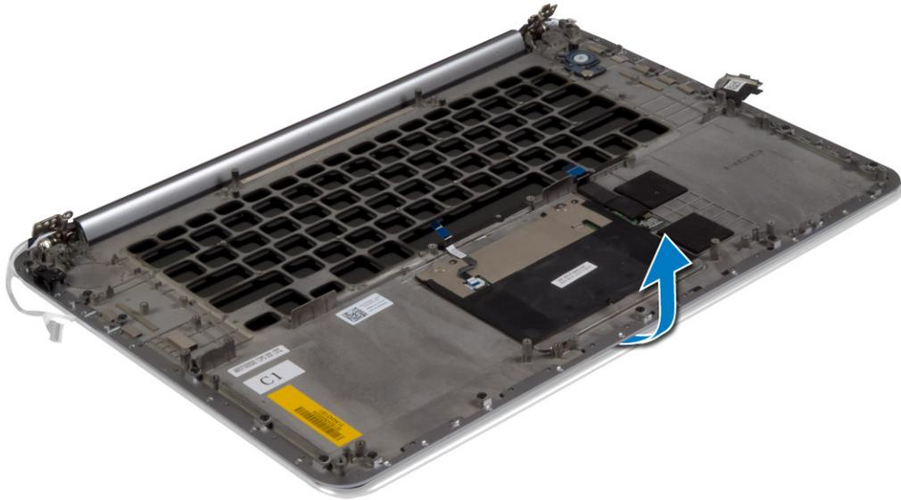
5. Remove the palmrest assembly away from the display assembly.
