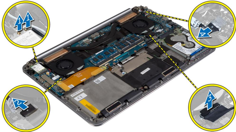
4. Remove the screws that secure the display hinges to the palmrest assembly.
