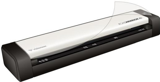
3. Place your thumbs on either side of the paper feed slot, underneath the lid of the scanner. Hold the scanner sides firmly and pull the scanner lid up to release it from the body of the scanner.
