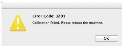
**Note:** if you attempted to calibrate the scanner with any page other than the calibration page provided with your scanner, the calibration routine will fail. You will need to power cycle the scanner, through unplug then re-plug of the USB cable, and then restart the calibration.
