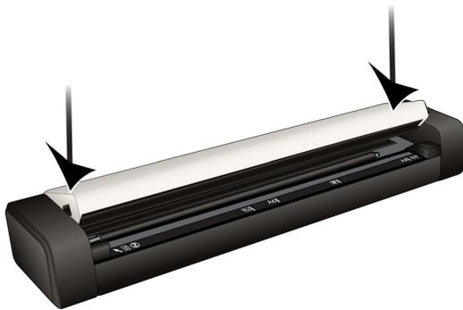
To reduce the number of paper jams, smooth and straighten the paper before scanning, and insert the paper evenly into the scanner.
