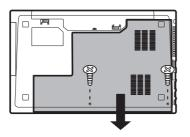
• Unplug two screws and open the back cover.
