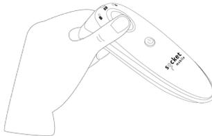
4. Keep holding the scan button until you hear a beep and then release (about 15 seconds). Your scanner will beep 5 times and power off.
