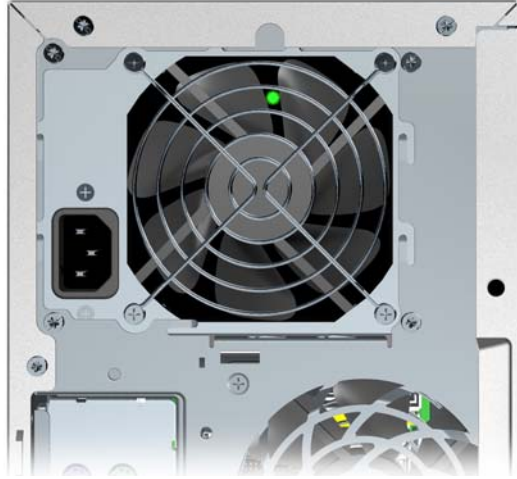
Figure 5-1 Testing power supply with BIST LED
