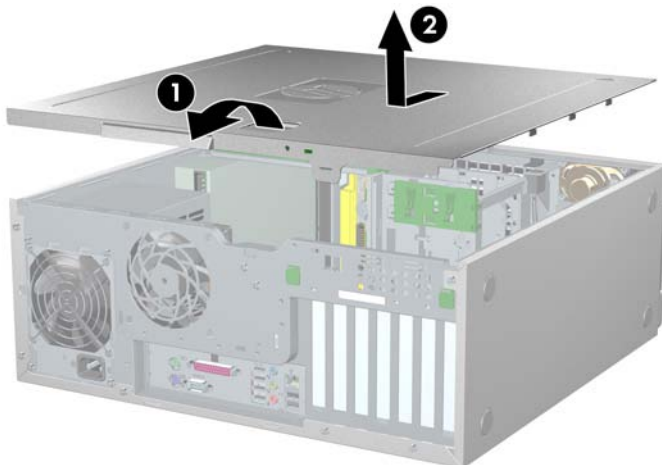
Figure 4-6 Opening the side access panel
