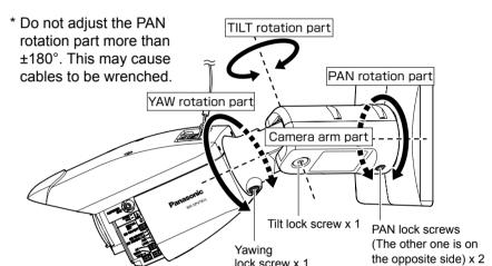
\* The front cover, including cables and wires, and Protection cover are not shown in the illustration
