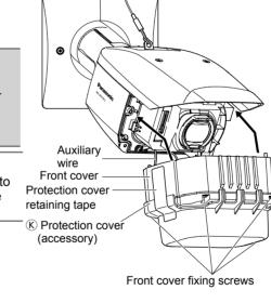
®Secure the H safety wire (accessory) to the ceiling or wall.
