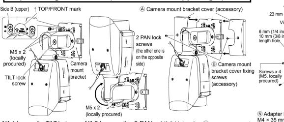
[1]-1 Loosen the TILT lock screw by about 1 turn until the camera faces downward and then temporarily tighten the TILT lock screw. After this, use the 2 upper M5 screws (locally procured) to
