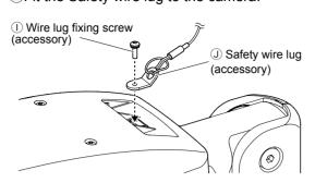
Recommended tightening torque: 0.6 N·m {0.44 lbf·ft}
