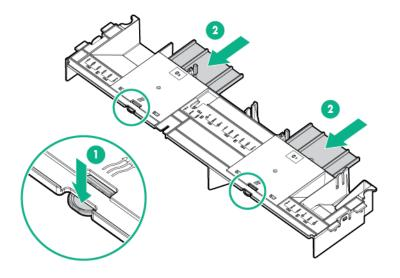
**b.** Install the appropriate retention clip onto the air baffle. Install the clip that supports your configuration. Primary, secondary, and tertiary positions are shown.
