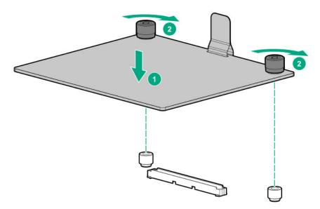
• For Type-p Smart Array controllers, install the controller in a compatible expansion slot.
