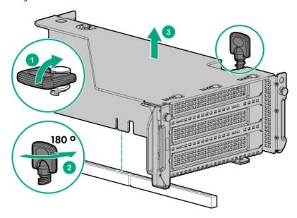
Remove the rear wall blank.
