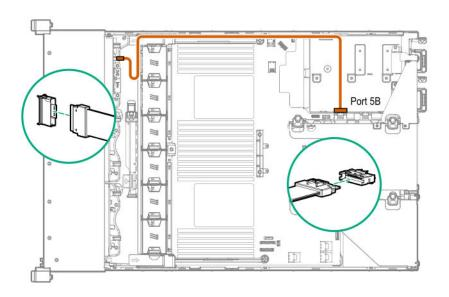
Cable routing: Front 2SFF NVMe drive option for LFF
