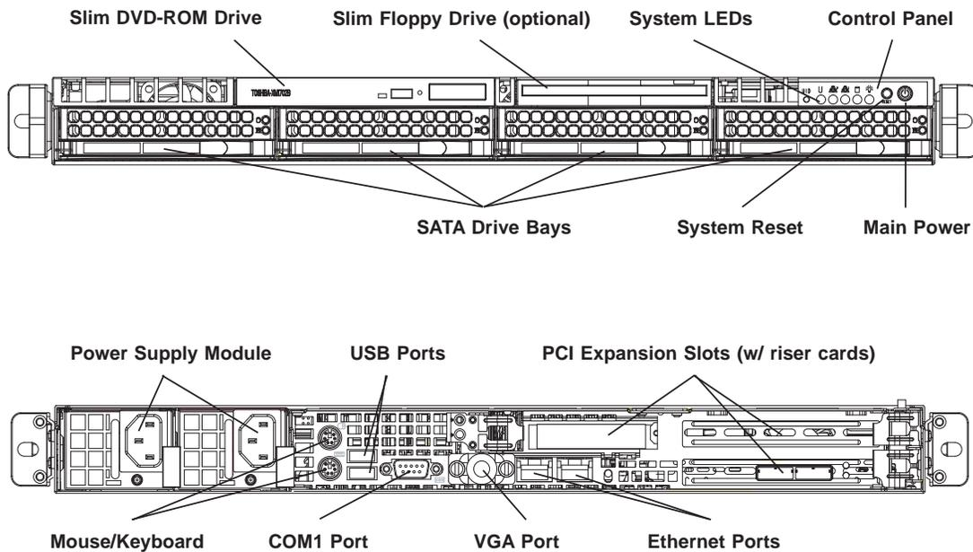
**Note:** the SC815TQ-560U chassis (6015C-U/6015C-NT) has only a single power supply module.
