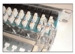
6. After terminating each pair, make sure the aluminum foil fully covers the wires.
