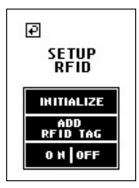
**Step 8:** Place the supplied RFID tag near the bottom right hand corner of the DL3<sup>™</sup> until you hear a "beep" tone.
