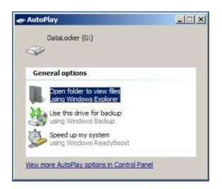
After you press the [CONNECT] button on the DL3<sup>™</sup> drive, it will begin connecting to the computer. By default, Windows will show an AutoPlay dialog once the drive has successfully connected.
