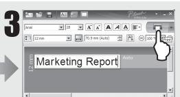
Enter the desired text and click the **Print** button. If **Auto Cut** is set to ON (default setting) in the **Print Options**, the tape will advance and cut your label to accommodate the small margins.
