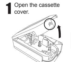
Verify that the P-touch labeller is turned off. Open the cassette cover as shown by the arrow in the above illustration while pressing the "<<" section of the tape cover.
