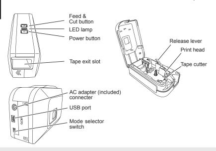
The PT-2430PC has 2 mode selector settings - "EL" and "E". The mode selector switch is pre-set at the factory to the EL mode, for use with P-touch Editor Lite. For E mode, you will need to install P-touch Editor 5.0, a more advanced labeling software, and the required drivers from the enclosed CD. For details on how to install P-touch Editor 5.0, see "Starting P-touch Editor 5.0" below.
