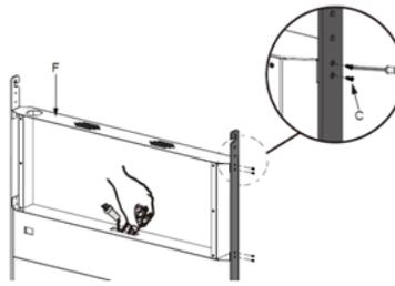
4. Secure the front cover of the device box (F) to the later with the included flat head screws (M3xL8) (C) by a Phillips screwdriver.
