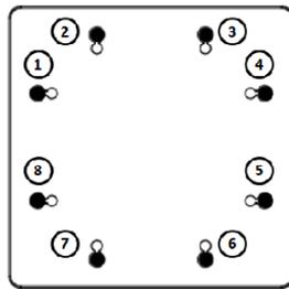
There are two loops of screw holes (outer & inner), depend on the design of each model. (Please check the user manual for using loop information)
