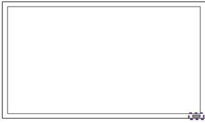
When using the remote control, make sure the display's remote control sensor window is **NOT** exposed to direct sunlight or strong reflected light, e.g. tile flooring.
