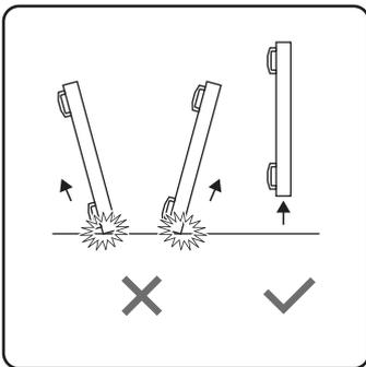
Be careful not to scratch any parts of the display when upturning the display.
