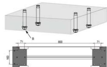
3. Hammer the expansion screws (M8xL60) (B) in the holes drilled earlier and tighten their nuts.
