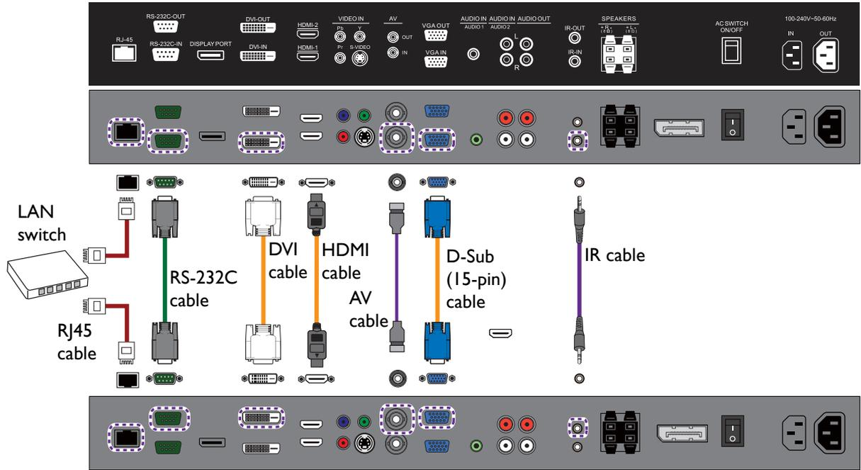
The first display (connected to the OUT ports)
