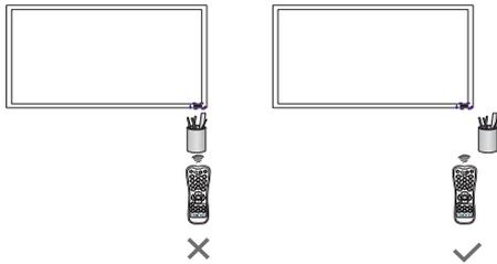
When using the remote control, confirm there is no object between the remote control and the remote sensor of the product.
