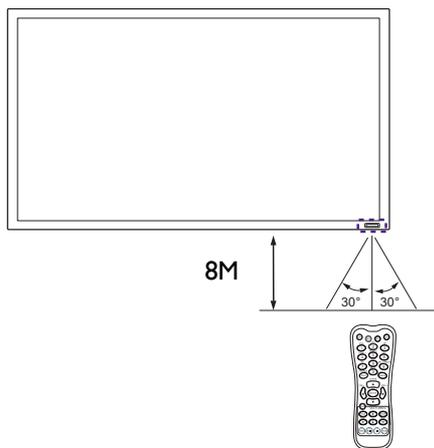
Operate the remote control from a location closer to the display's remote control sensor window. Adjust the distance between the remote control and the display.
