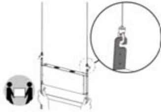
2. Secure the bracket to the panel display with the included flat head screws (M4xL10) (D) by a Phillips screwdriver.
