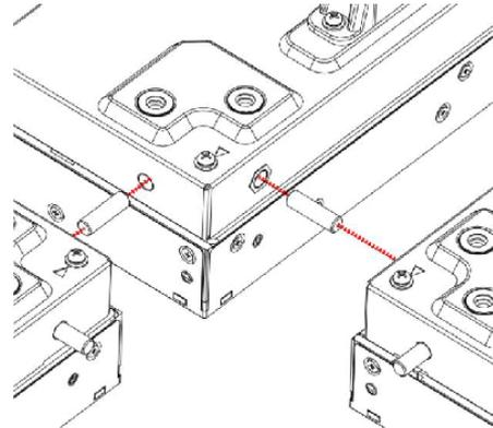
There are 8 holes on the four corners of displays designed for plug-in the edge alignment pin.
