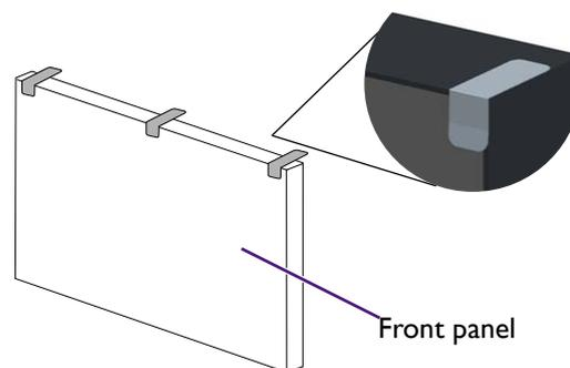
4. After the displays are mounted and fastened, check if the space between each display is just enough for removing the gap inspection pad smoothly. If the pad is trapped, adjust the screws to release more space.
