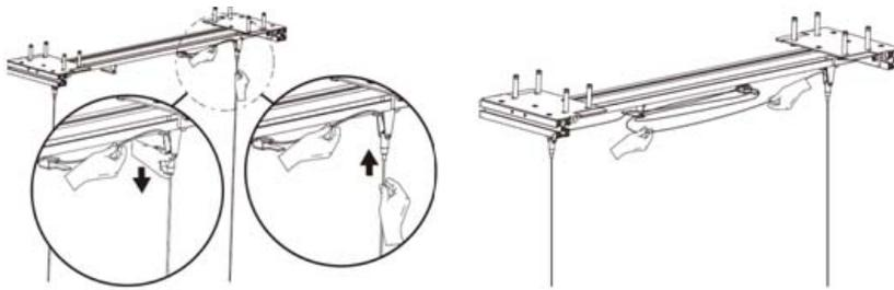
2. Replace the plastic covers to the left and right of the bracket before securing them with the included flat head screws (M3xL8) (C) by a Phillips screwdriver.
