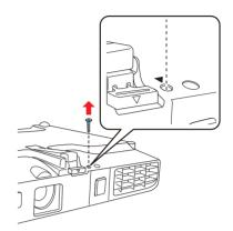
Remove the wireless LAN module cover.
