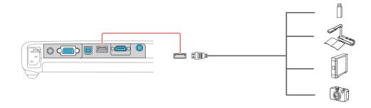
If you connect a digital camera, USB flash drive, or USB storage device, you can use the projector's Slideshow feature to project images. See the online *User's Guide* for details.
