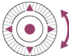
3. Select the desired setting item by pressing the up/down/left/right side on the control wheel or by turning the control wheel, and then press
