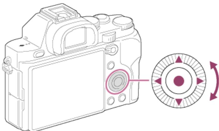
When you turn or press the top/bottom/right/left side of the control wheel, you can select setting items. Your selection is determined when you press ● on the center of the control wheel.
