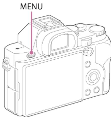
2. Select the desired MENU item using the up/down/left/right side of the control wheel or by turning the control wheel, and then press
