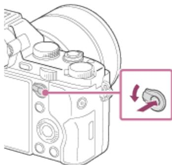
The exposure is locked, and
