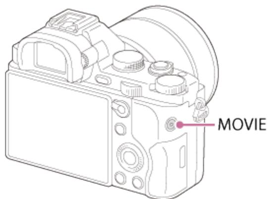
To adjust the shutter speed and aperture value to the desired settings, set the shooting mode to
