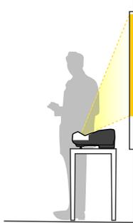
Rear projection from a table or portable cart behind a translucent screen (interactive features not supported)
