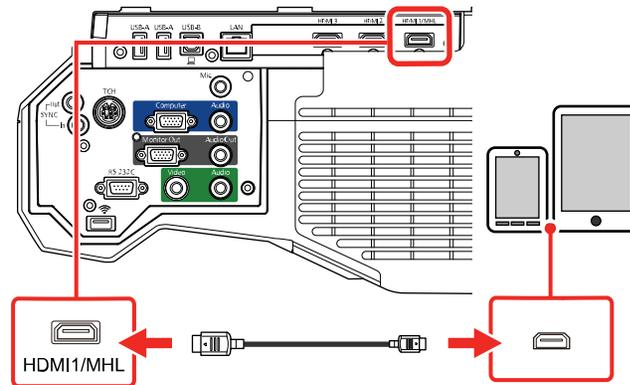
**Note:** The projector converts the digital audio signal sent from your video source into a mono analog signal for the internal speaker or a stereo analog signal if you are connecting to external speakers.
