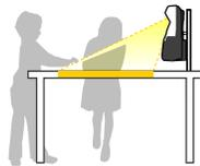
Mounted on the wall or ceiling and projecting from behind a translucent screen (interactive features not supported)
