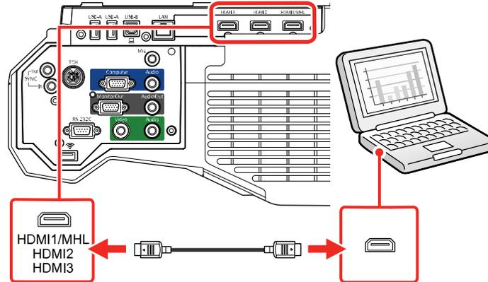
**Note:** The projector converts the digital audio signal sent from your computer into a mono analog signal for the internal speaker or a stereo analog signal if you are connecting to external speakers. (Make sure the HDMI audio playback device on your computer's audio settings is set to **EPSON PJ.**)
