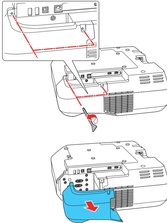
To attach the cable cover, slide it into position and tighten the screws with a screwdriver.
