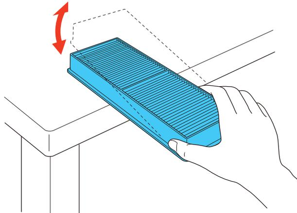
**Caution:** Do not use excessive force when tapping the air filter, or it may crack and become unusable. Do not rinse the air filter in water, or use any detergent or solvent to clean it. Do not use
