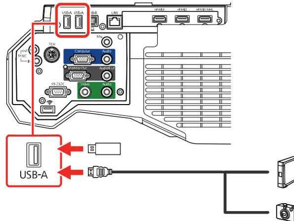
**Note:** Do not connect a USB hub or a USB cable longer than 10 feet (3 m), or the device may not operate correctly.
