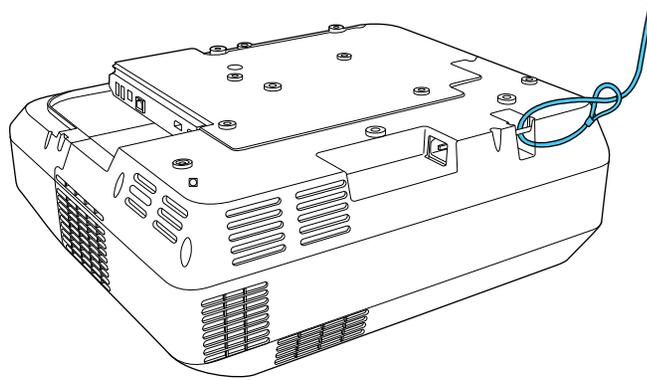
**Note:** Do not pass drop-prevention cables through the security cable attachment point when mounting the projector on a wall or ceiling.
