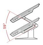
After tilting your computer back, you can adjust the UltraFlex II Stand downward by up to 59°.
