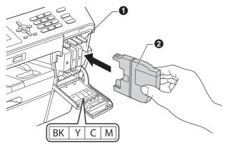
Gently push the back of the ink cartridge marked "PUSH" until it clicks. After all the ink cartridges are installed close the ink cartridge cover.
