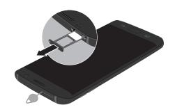
Slide the SIM card/Memory card tray back into the slot.
