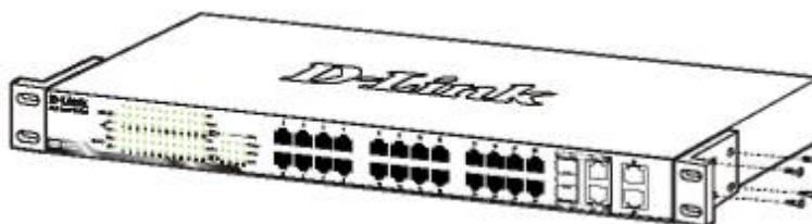
Figure 2.2 – Attach the mounting brackets to the Switch
