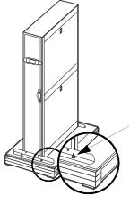
3 Remove the bolts securing the transport brackets to the pallet on the front and back of the enclosure.
