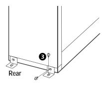
3 Attach the stabilizing brackets to the back of the enclosure with screws and washers (provided). Attach screws for floor anchoring (not provided).
