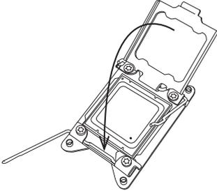
**2** Push down and lock the lever labeled 'Close 1st'.
