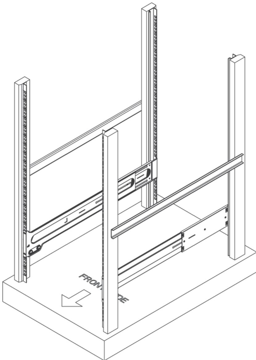
3. Slide the chassis rails into the rack rails, keeping the pressure even on both sides (you may have to depress the locking tabs when inserting). When the server has been pushed completely into the rack, you should hear the locking tabs "click" (Figure 2-7).
