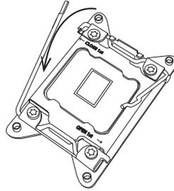
2. With the lever labeled 'Close 1st' fully retracted, gently push down on the lever labeled 'Open 1st' to open the load plate. Lift the load plate to open it completely.
