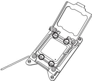
**Warning:** You can only install the CPU inside the socket in one direction. Make sure that it is properly inserted into the CPU socket before closing the load plate. If it doesn't close properly, do not force it as it may damage your CPU. Instead, open the load plate again to make sure that the CPU is aligned properly.
