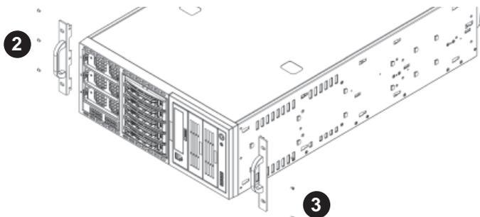
2. Align the chassis handle with the front of the chassis and secure with the three chassis handle screws.
