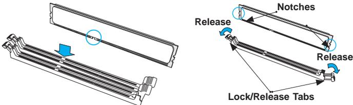
3. Align the key of the DIMM module with the receptive point on the memory slot.
