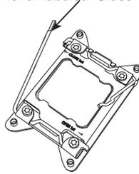
8. Close the load plate with the CPU inside the socket. Lock the lever labeled 'Close 1st' first, then lock the lever labeled 'Open 1st' second. Using your thumb gently push the load levers down to the lever locks.
