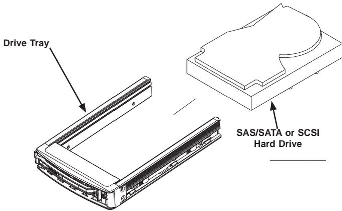
5. Secure the hard drive to the tray using four screws (Figure 6-13).
