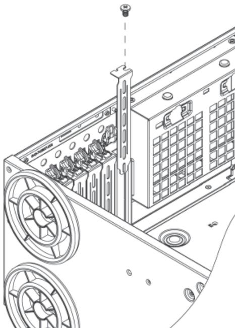
5. Install your PCI card or other add-on card into the PCI slot bracket and serverboard. To do this, slide the PCI card (with "L" bracket) into the PCI slot and secure the card to the serverboard.
