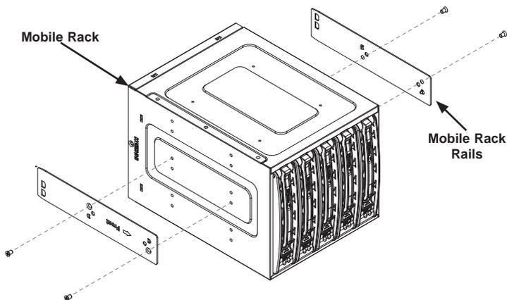
5. Slide the mobile rack into the chassis.
