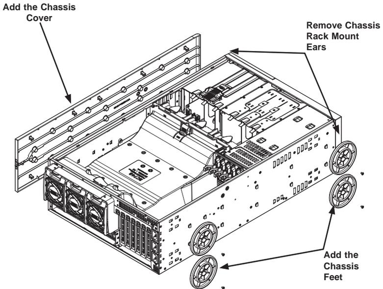
2. Align the cover post with the corresponding holes on the top of the chassis and place the cover on top of the chassis. The cover should overhang
