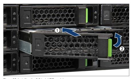
Figure 35: Installing the 3.5-inch HDD module
