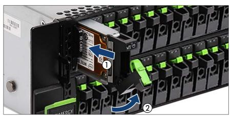
Figure 41: Installing the EDSFF SSD module
