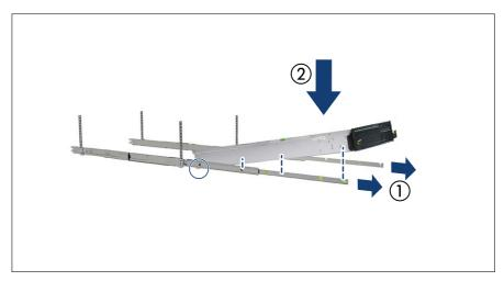
Figure 23: Installing the server in the rack rails
