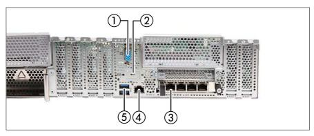
Figure 16: Connectors on the server rear
