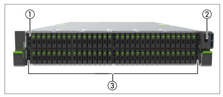
Figure 5: Front side 64x EDSFF SSDs
