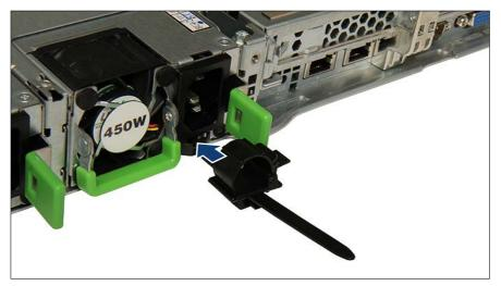
Figure 45: Installing the cable clamp
