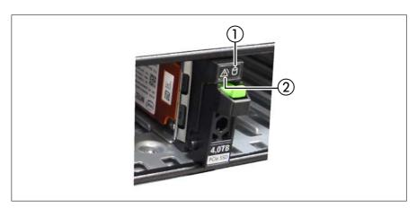
Figure 15: Indicators on an EDSFF SSD module
