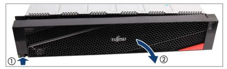
Figure 32: Removing the front cover
