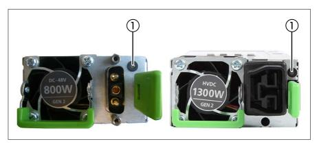
Figure 21: PSU status indicator (DC PSU)
