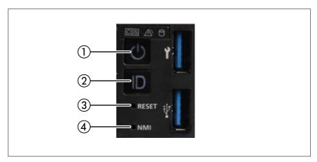
Figure 11: Controls on the COP
