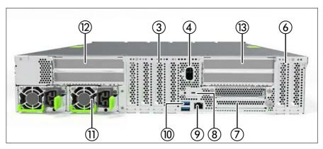
Figure 8: Server rear (configuration with riser modules)
