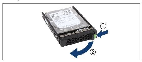
Figure 37: Opening the locking lever
