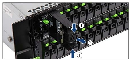
Figure 39: Removing an EDSFF dummy module
