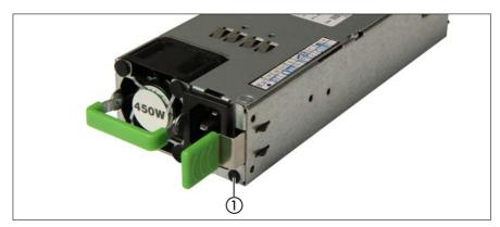
Figure 20: PSU status indicator (AC PSU)
