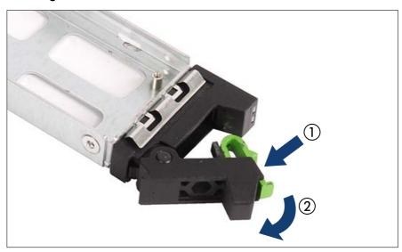
Figure 40: Opening the locking lever
