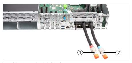
Figure 17: Quick connectors for liquid cooling
