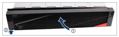
Figure 29: Installing the front cover with lock
