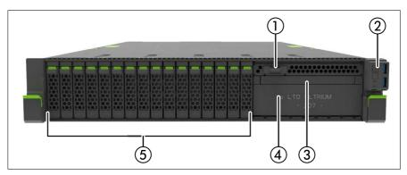
Figure 3: Front side 16x 2.5-inch HDDs / SSDs / PCle SSDs
