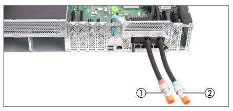
Figure 25: Quick connectors for LC
