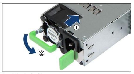
Figure 44: Installing the PSU
