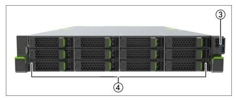
Figure 2: Front side 12x 3.5-inch HDDs
