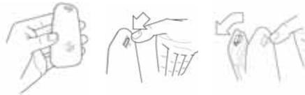
The keypad lifts out from the back of the device, as shown in the diagram. Take care not to drop the keypad.
