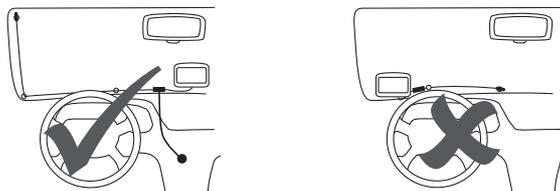
4. Then place the remaining suction cups along the edge of the windshield, as shown, and keep the cable straight.
