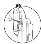
4. Place the crevice tool /dusting brush into the tool holder.
