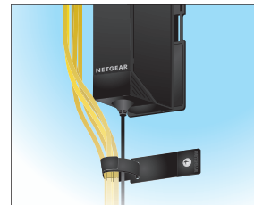
Strap the cables to the wall
