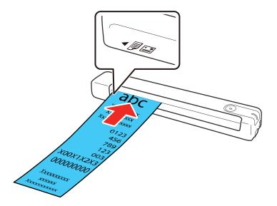
• For envelopes, slide the original into the input slot against the left side as shown until it meets resistance. Make sure the printed side is faceup and the flap is facing as shown. For envelopes with the flap on the shorter side, load the envelope with the flap side last.
