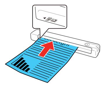
For longer originals, slide your original into the input slot against the left side as shown until it meets
