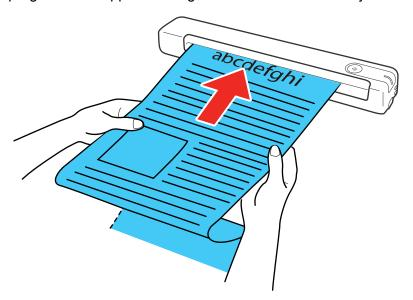
• For receipts, support the original by hand and load it into the input slot against the left side as shown until it meets resistance. Make sure the printed side is faceup and top edge first.
