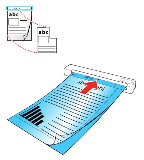
**Note:** Only use the carrier sheet designed for your scanner. If the carrier sheet is scratched or has been scanned more than 3,000 times, stop using it and obtain a new one.
