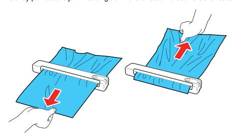
**Note:** If paper gets stuck in the roller and remains inside the scanner, carefully remove it with a pair of tweezers in the direction of the output slot. If you cannot remove it, contact Epson for support.
