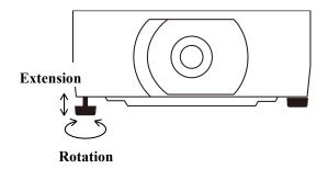
Rotate the adjustable feet to adjust their lengths.
