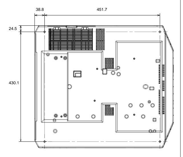
These screw holes normally have adjustable feet attached to them. If the product is to be suspended from the ceiling, the adjustable feet need to be removed.
