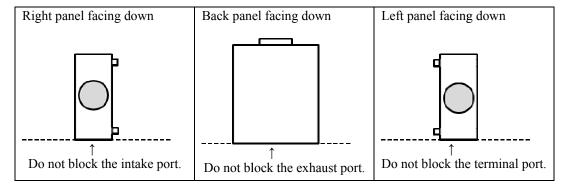
If the product is to be installed in a special orientation, a safe and stable installation method needs to be considered by a specialist.
