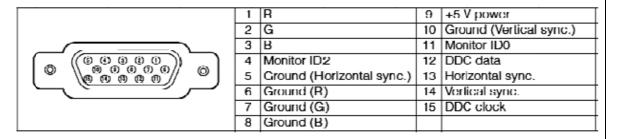
A cable with conduction lines for Nos. 9, 12, and 15 is necessary.
