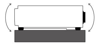
The front-to-back angle of this product can be adjusted in the range of  $\pm 1.8$  degrees relative to the surface that the product is placed on.
