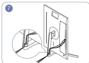
7 Place the corresponding cables into the stand-neck holder. Do not stretch the line. Three cables in one holder is recommended.
