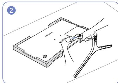
To disassemble the stand from the monitor, make sure to press the lower part of the monitor with one hand, and pull and sway sideways the stand with the other hand, as shown in the picture.
