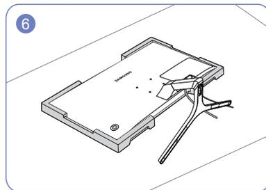
Install the COVER-REAR SUB after the power supply and the data cable are connected.
