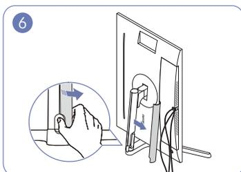
6 Open the COVER-STAND NECK LEFT, and rotate the open part at the bottom.
