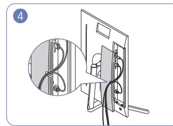
4 Arrange the cables against the bend tendency of the cables and pull the cables out of the COVER-REAR SUB grooves.
