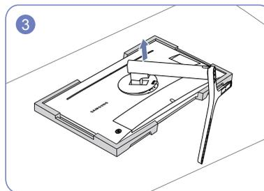
After turning the stand neck of the display counterclockwise for 10°, lift the stand neck to detach it from the device.
