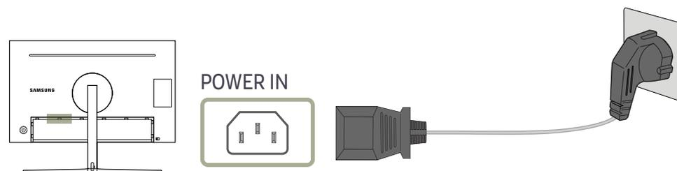
To use the product, connect the power cable to a power outlet and the **POWER IN** port on the product.
