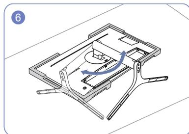
Turn the stand neck of the display clockwise for 90° to ensure that the stand neck of the display is put into place.
