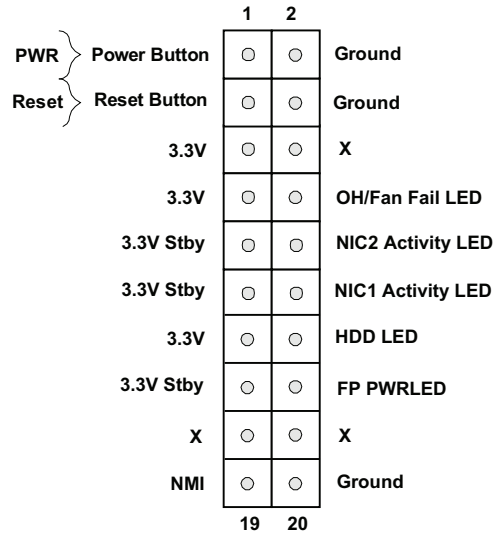
Figure 3-1. JF1: Control Panel Pins
