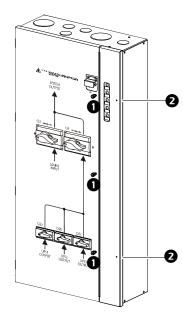
3 Use a knockout punch to create appropriate-sized holes for the cables/conduits (38 or 76 mm) in either the top or bottom plates of the MBP.
