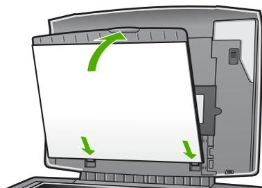
3. Place the bottom notch of the Slide and Negative Film holder under the tab at the right bottom corner of the lid.
