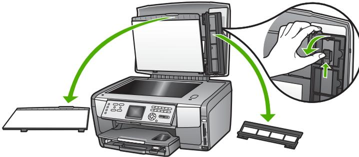
2. Unfold the holder so that the negative film portion is on top and the film opening is on the right side.
