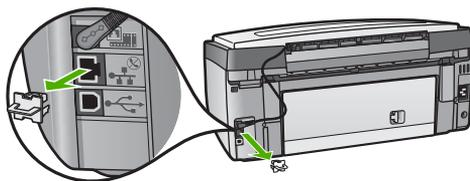
2. Connect the Ethernet cable to the Ethernet port on the back of your HP All-in-One.
