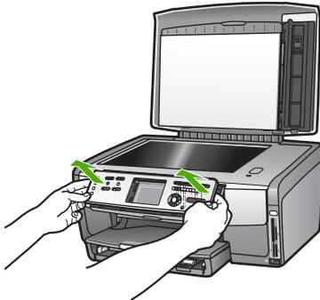
2. Retain the control panel faceplate. Do not return the control panel faceplate with the HP All-in-One.
