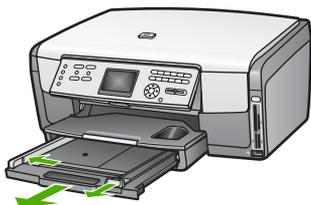
3. Insert the stack of cards into the far right side of the main tray with the short edge forward and the **print side down**. Slide the stack forward until it stops.
