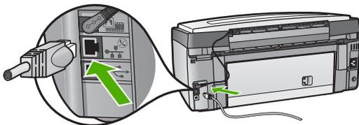
3. Connect the other end of the Ethernet cable to an available port on your Ethernet router, switch, or hub.
