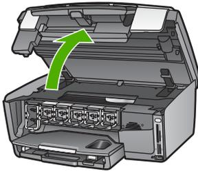
3. Squeeze the tab below an ink cartridge to release the latch inside the HP All-in-One; then lift the latch.
