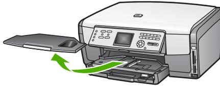
2. Insert the stack of photo paper into the photo tray with the short edge forward and the **print side down**. Slide the stack of photo paper forward until it stops.
