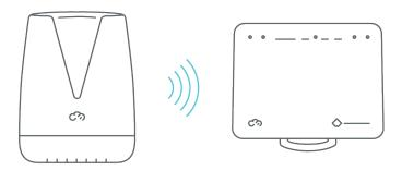
Press and release the **WPS button** on the **Satellite**, then press and release the **5G WPS button** on the **Gateway** within **two minutes**.
