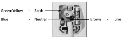
If you change the plug, the colour of wires in the mains lead may not correspond with the colour of the markings identifying terminals in the plug. You should therefore wire it as shown above.
