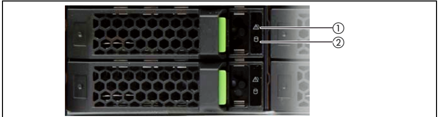
Figure 16: Indicators on the 3.5 inch HDD modules
