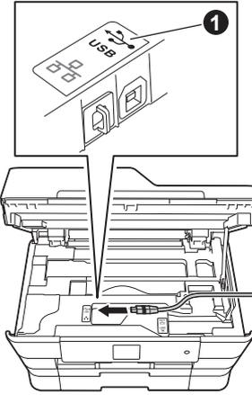
**c** Carefully guide the USB cable into the cable channel and out the back of the machine. Connect the cable to your Macintosh.
