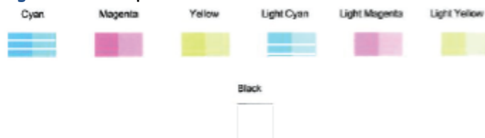
Figure 9-2 Example of color blocks with defects
