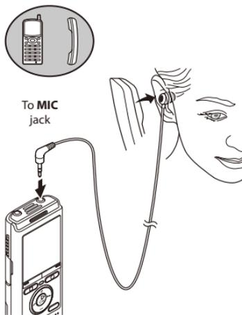
Example: TP8 telephone pickup microphone (optional)
