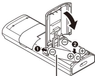
Insert the battery's negative terminal first
