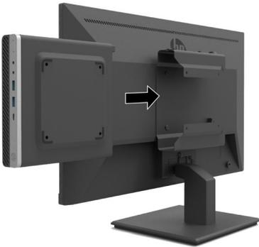
3. Install the DT Mini PC to the Dual VESA Sleeve V2.
