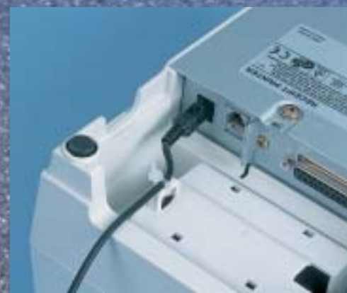
Optional Power Connection Security Tie Strap
