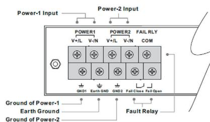
Figure 3-7. Redundant power inputs.
