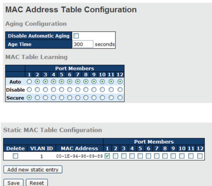
Figure 5-103. MAC Address Table Configuration and Static Mac Table Configuration screens.
