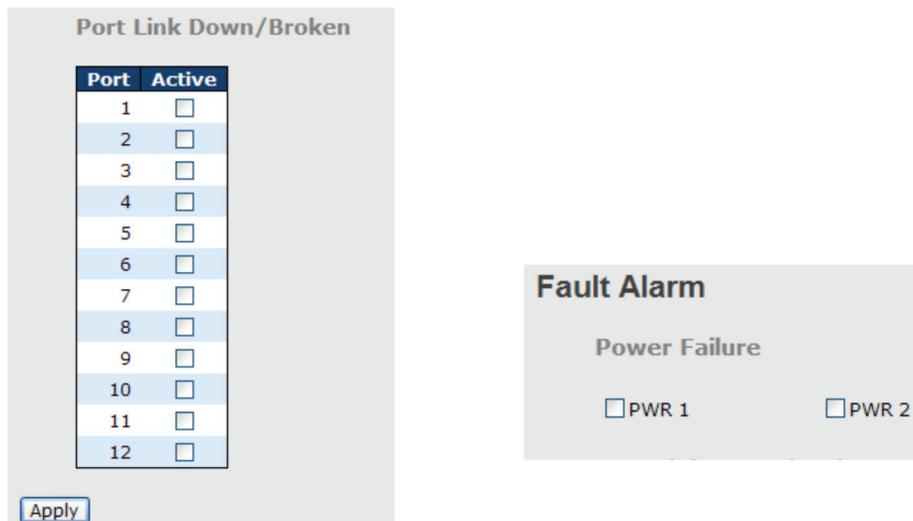
Figure 5-99. Port Link Down/Broken and Fault Alarm screens.
