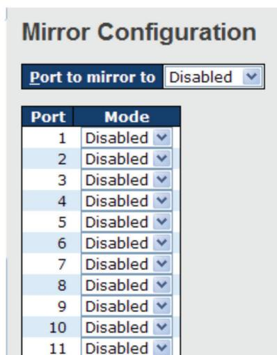
Figure 5-109. Mirror Configuration screen.
