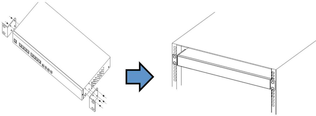
Figure 3-1. Installing the module.
