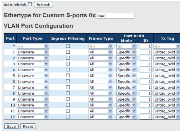
Figure 5-33. VLAN Port Configuration screen.
