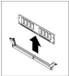
4. Position the new memory module over the memory connector. Make sure that the notch 1 on the memory module aligns correctly with the connector key 2 on the system board. Push the memory module straight down into the connector until the retaining clips close.
