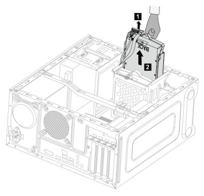
4. Remove the hard disk drive from the plastic bracket as shown.
