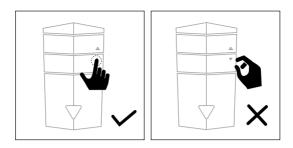
Press the arrow button at the top right of the case to open the front I/O door. Do not force the door open. Press the arrow button again to close the door.
