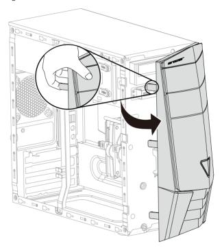
3. To reattach the bezel, align the plastic tabs on the bottom of the bezel with the corresponding holes in the chassis, and then snap it into position.
