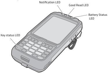
The next table describes the notification LED, Good Read LED, and key status LED. For information about the battery status LED, see "Understanding the Battery Status" on page 6.
