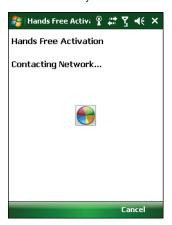
**2** If activation is unsuccessful on the first attempt, the wizard will countdown from 60 seconds and try again. It will continue this process four times before it stops. At this point, you can reboot the CN50 to retry activation or contact Intermec Support.
