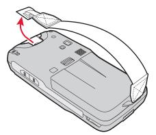
Push forward on the battery release tab until the battery releases, and then lift it away from the CN50.
