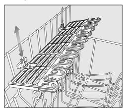
Slide the glass rack to the desired height until the catches click into place at the top or rest on the bottom.
