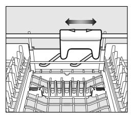
You can use the yellow slide to adjust the height of the middle section of the cutlery tray to make more room for large items of cutlery, such as serving spoons and ladles. Both rows of spikes in the middle section of the cutlery tray can be flipped over to make room for larger pieces of cutlery.
