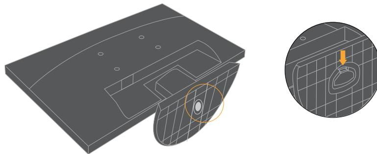
2. Strip down the screws by Anti-clockwise direction, remove the stand and then assemble the VESA frame through VESA holes.
